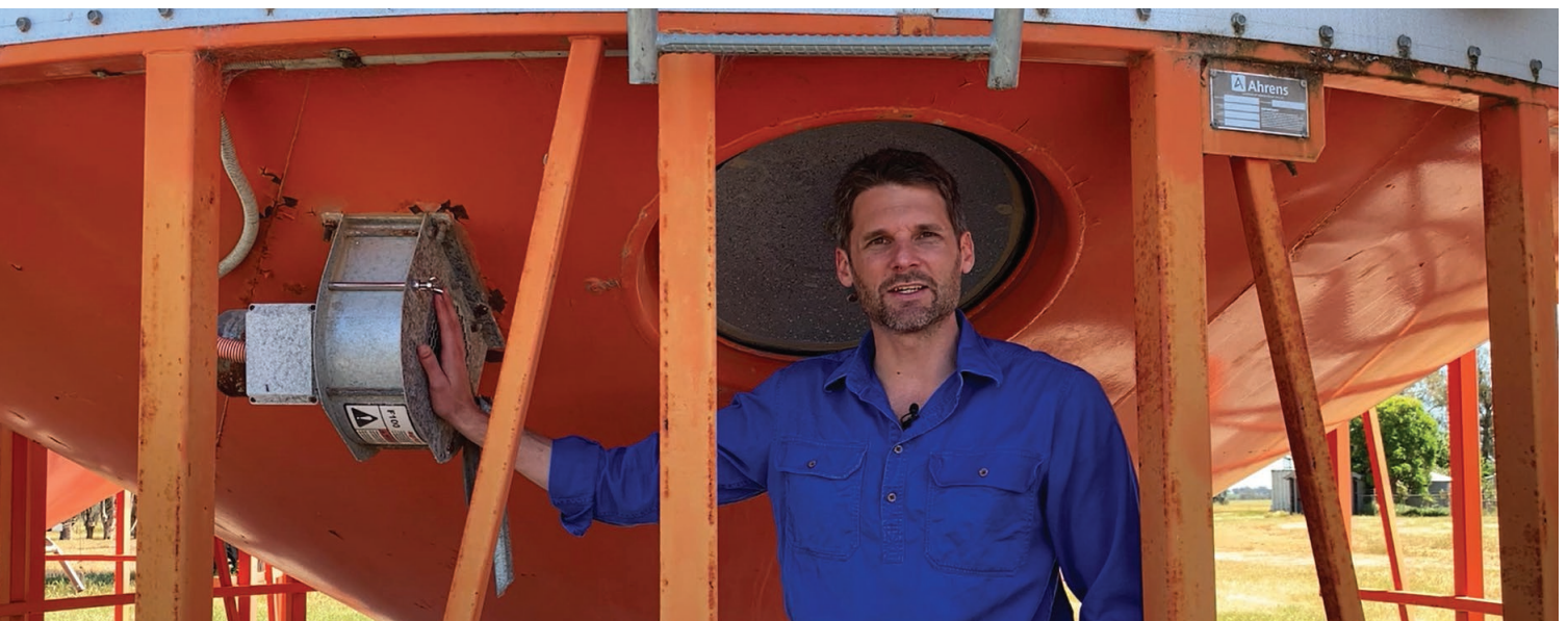
Chris Warrick says aeration cooling allows grain that was harvested slightly over moisture to be stored for up to three to four weeks before it is dried or blended with dry loads. (PHOTO:Chris Warrick)
