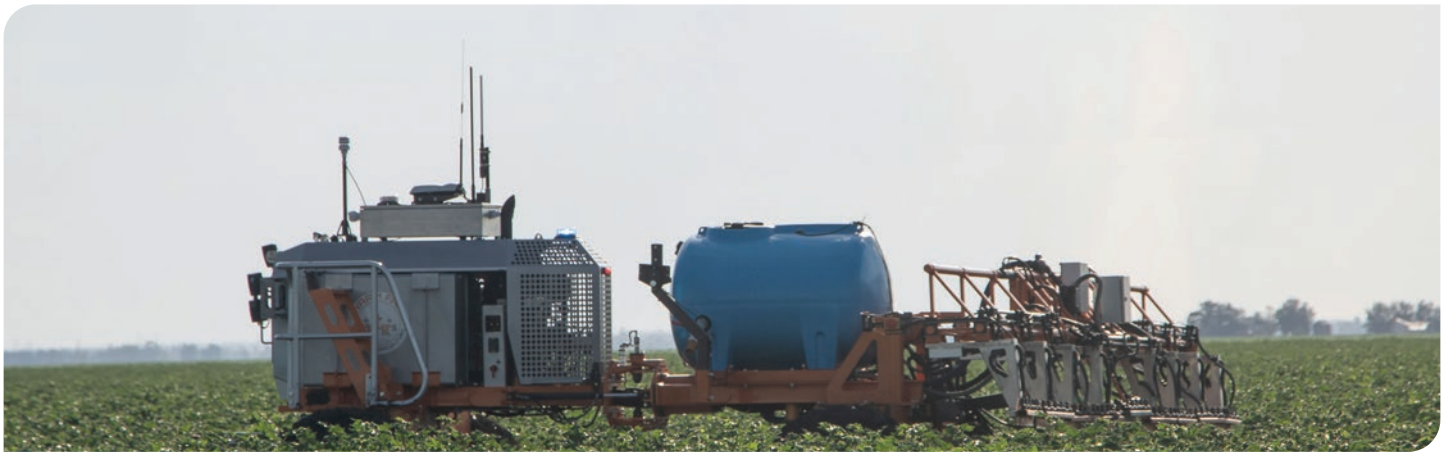
The robots work at a slow, steady pace, providing a stable platform for the boom and enabling the sensors to pick up weeds 5 mm in diameter. (PHOTO: Cindy Benjamin)
