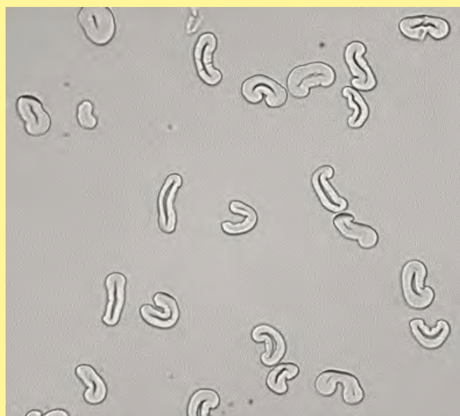
FIGURE 1: Cross-sections of cotton fibres embedded in methyl-butyl methacrylate resin showing variation in fibre cell wall and lumen
