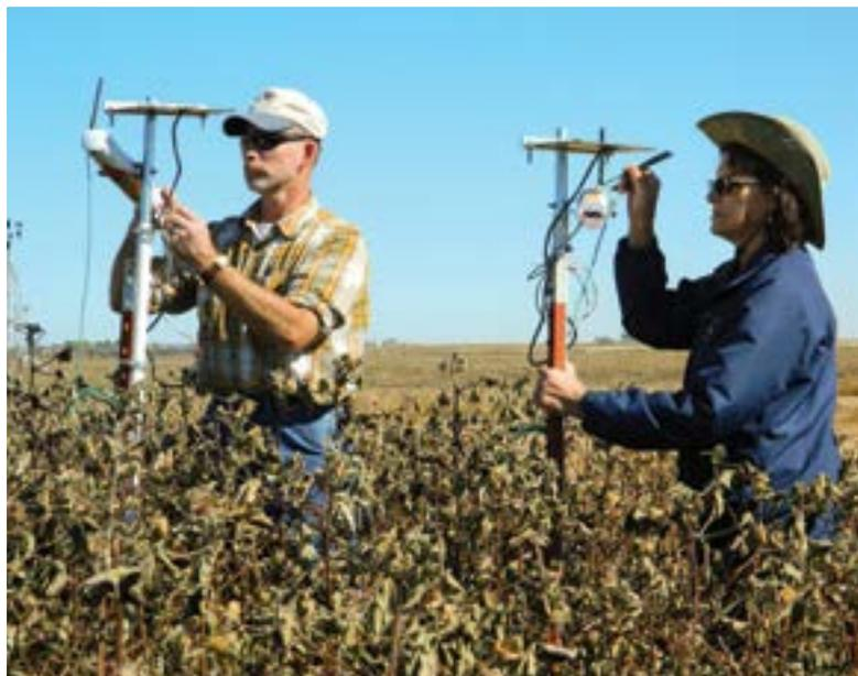
ARS agricultural engineers Susan O'Shaughnessy (right) and Paul Colaizzi adjust commercial wireless infrared thermometers that measure plant leaf and soil temperatures. (PHOTO: John Blundell)
