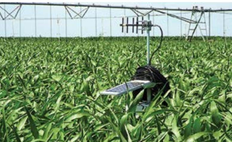
**Solar-powered soil water station in a corn field helps to prevent over- and under-irrigation of the variable-rate irrigation system. (PHOTO: Nancy Davis)**
