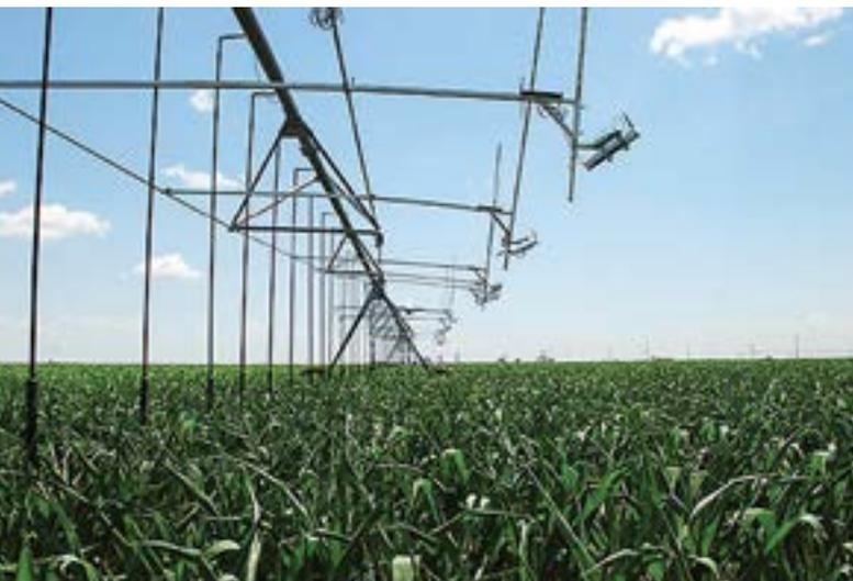
**Variable-rate irrigation sprinkler at Bushland, Texas, equipped with on-board canopy temperature sensors designed by ARS and commercialised by Dynamax, Inc. (PHOTO: Nancy Davis)**
