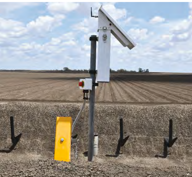
An EnviroNode siphon controller. (PHOTO: Lou Gall)
