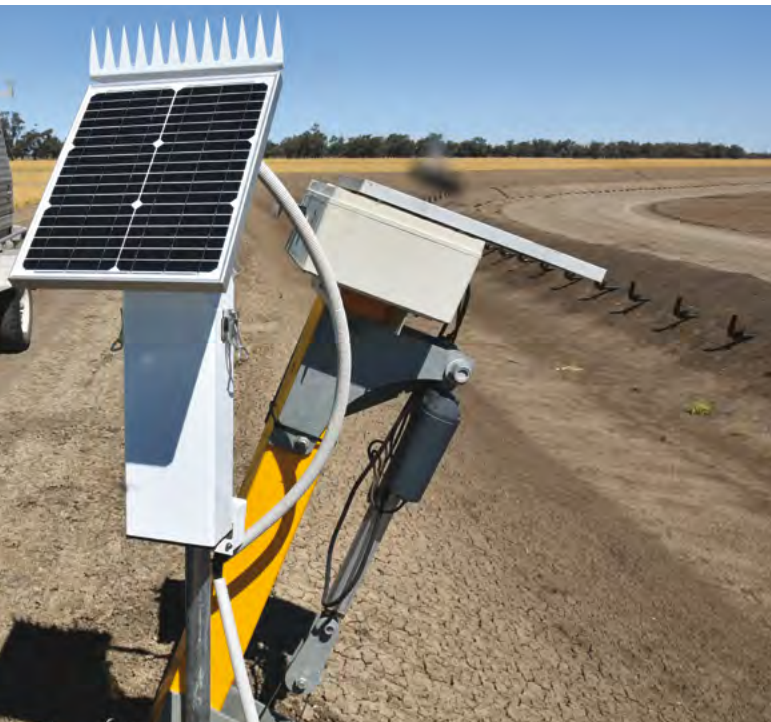
EnviroNode IoT control for Smart Siphons. (PHOTO: Lou Gall)
