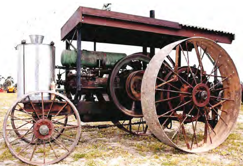
A 1917 Jelbart, made in Ballarat. Note the horizontal stepped cylinder. Owned by Tony Pailthorpe of Kukerin. (PHOTO: IMJ)
