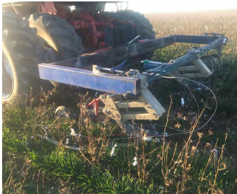
**Photo 4: The engagement tool is designed to ensure that each ratoon along the row has good exposure to the Mach 3 jet-stream.**
