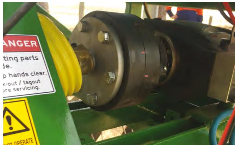
**Photo 2: A PTO drive version of the 50HP 50,000 psi Flow pump deployed in sugarcane as a liquid couler.**
