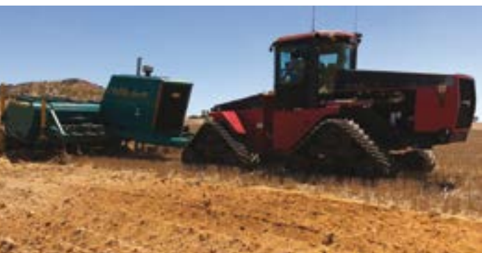
The Armadillo spader in action doing trial strips on 'Moonyoonooka', the property of our district reporter, Peter Norris. A 400 plus horsepower Cummins engine drives the two spader rotors that are each 3 metres wide giving a 6 metre cut. The machine is ripping to around 450 mm and spading to 350 mm.
