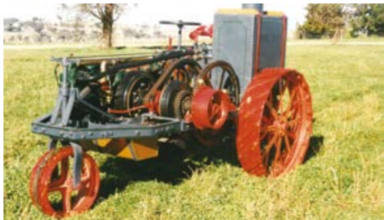
A view of Norm McKenzie's Ivel illustrating the drive mechanism. (Photo IMJ)
