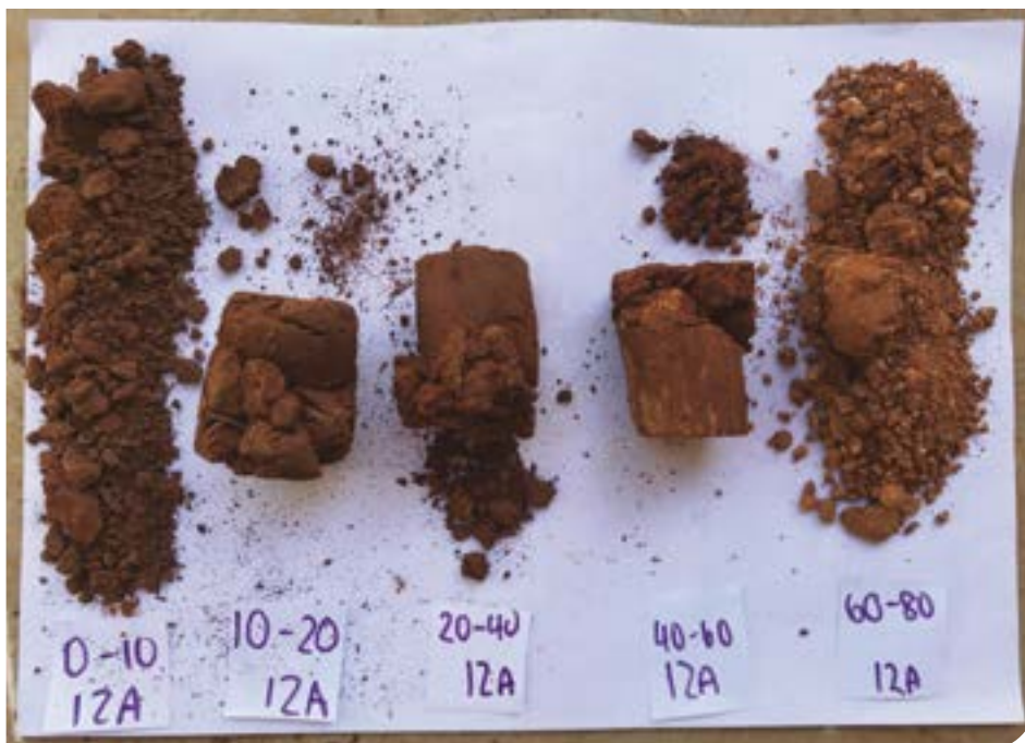
Soil moisture profile samples were taken at various depths up to 80 cm.
