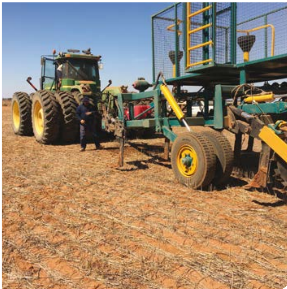
A Nufab ripper was used for incorporating gypsum in the first year of the MIG sodic soils trial.
