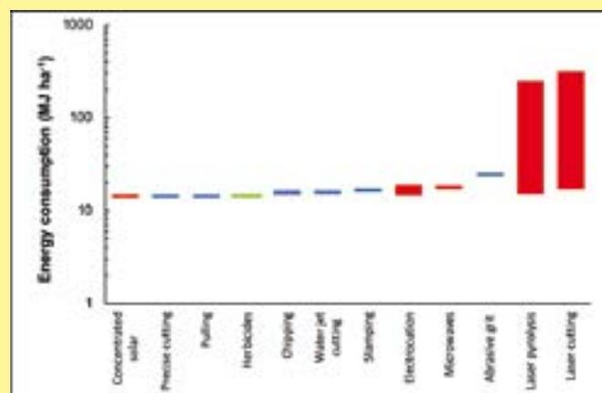
These values include the 14.4 MJ/ha used for image processing and weed detection. Mechanical treatments (blue bars), thermal treatments (red bars), herbicides (green bar). Source: G. Coleman.
