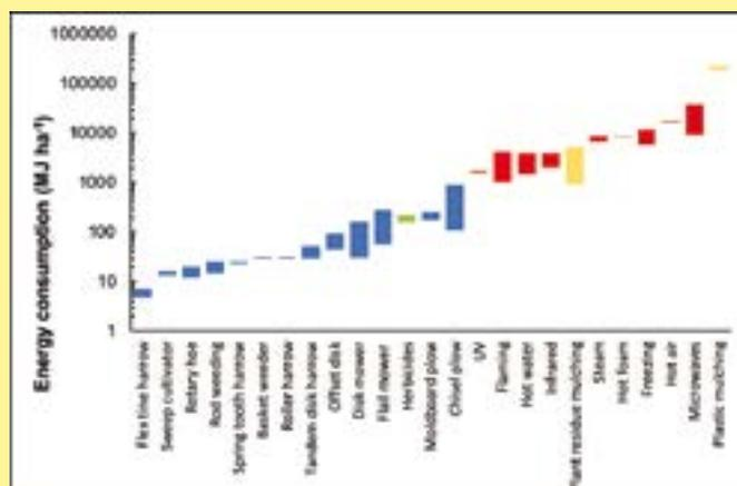
Mechanical treatments (blue bars) generally had much lower energy requirements than the thermal treatments (red bars). Herbicides (green bar), mulching (yellow bar). Source: G. Coleman.
