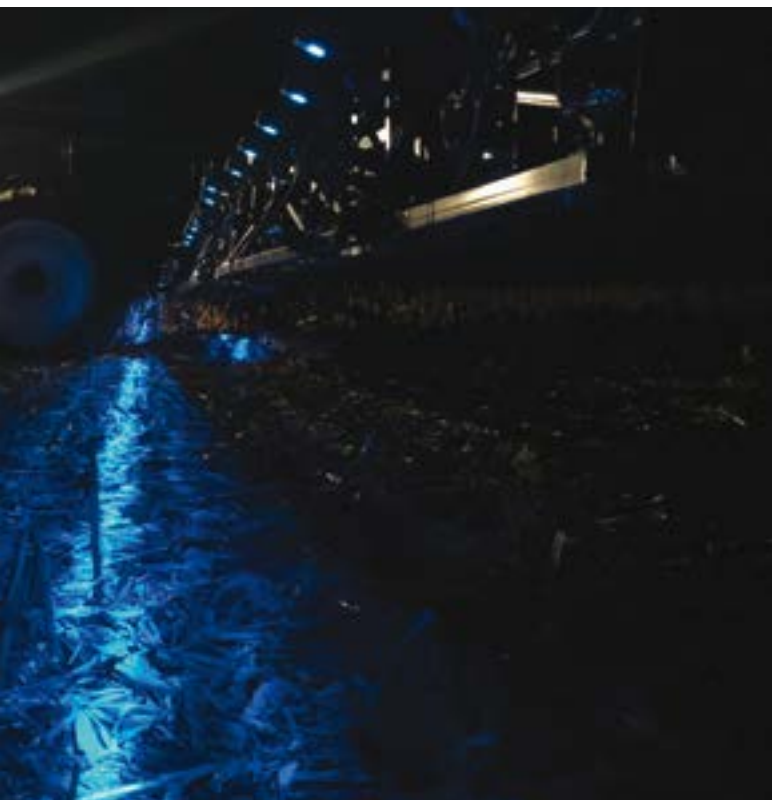
New blue light source is more sensitive to weeds and less sensitive to 'background noise'.
