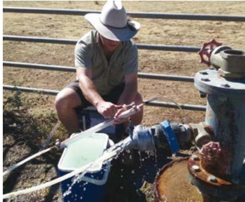
Sampling groundwater from an artesian stock bore screened in the Poole Sandstone aquifer of the Fitzroy catchment.
