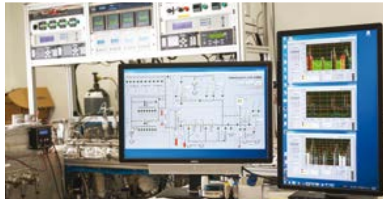
The first noble gas machine in the Southern Hemisphere, capable of analysing fossil water unique to Australia. (IMAGE: CSIRO/James Knowler)
