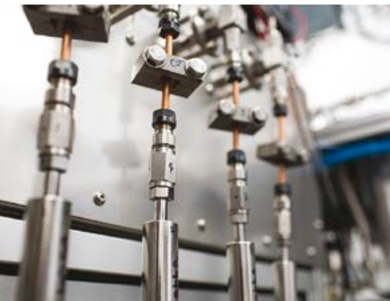
The copper tubes contain the gas extracted from water samples and, here, attached to the mass spectrometer for analysing. (IMAGE: CSIRO)
