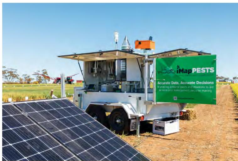
**The Sentinel, a mobile surveillance unit offers optimal sampling of airborne fungal spores and insects.**
