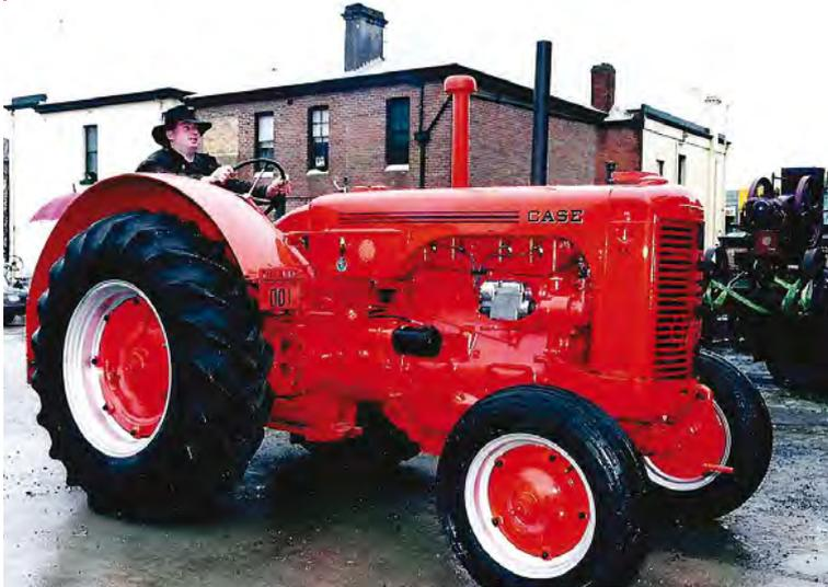
**This 1949 Case LA was considered one of the most powerful tractors in its day. The big four cylinder 403 cubic inch petrol/ kero fuelled engine produced a lazy 58.3 hp. Beautifully restored by Chris Broers. (PHOTO: IMJ)**
