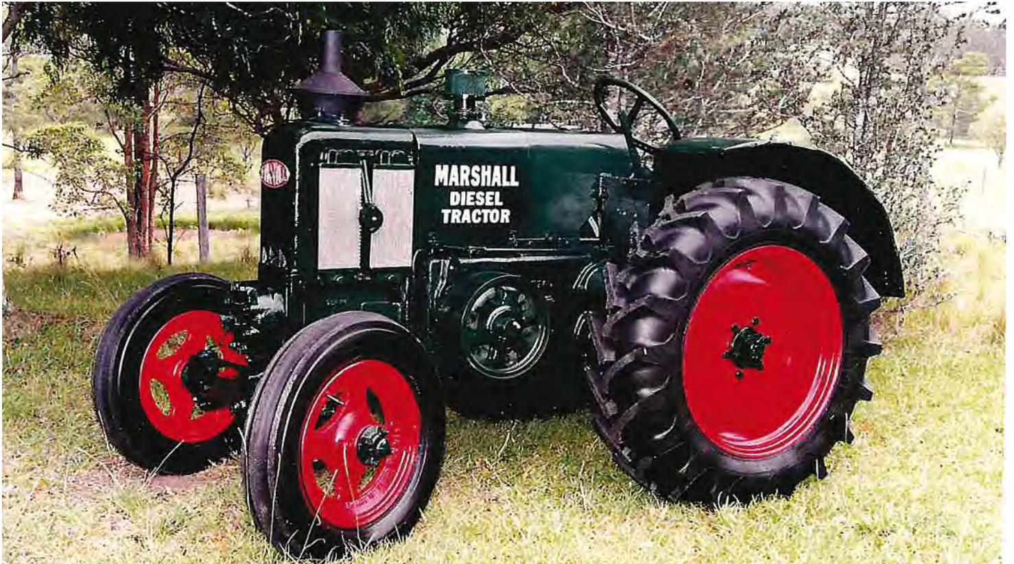
One of the restored gems in the author's collection was this 40 hp 1935 Marshall 12/20. Only a total of 200 were produced. Although having only a single cylinder, it differed from Lanz tractors by being a full compression diesel. Starting was by an igniter and hand crank of the flywheel. (PHOTO: IMJ)
