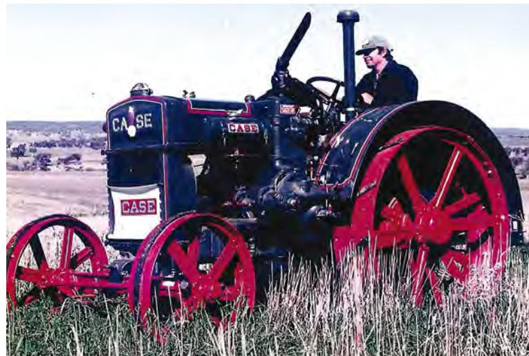
This magnificent example of a 1929 Case 18/36 was restored by Norm Mackenzie. The 4 cylinder engine was mounted east/west immediately ahead of the operator, with its open exhaust blasting heat, fumes and noise in front of his face. (PHOTO: IMJ)
