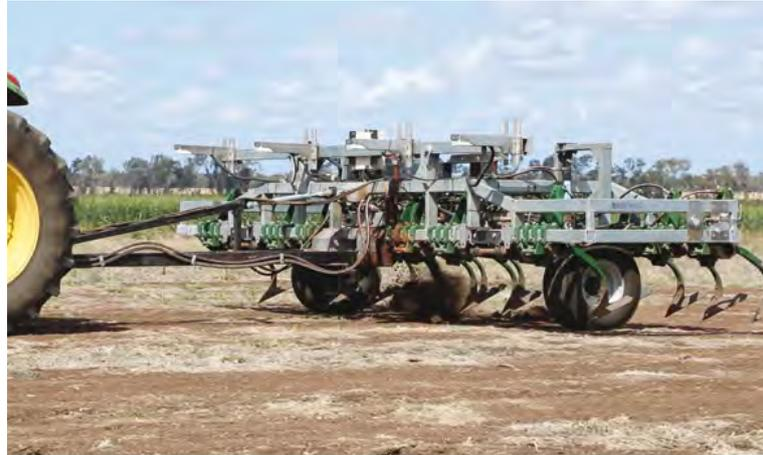
The WeedChipper uses sensors to detect weeds and activate a tyne that can dig out large plants or weeds that are difficult to kill using current herbicides.
