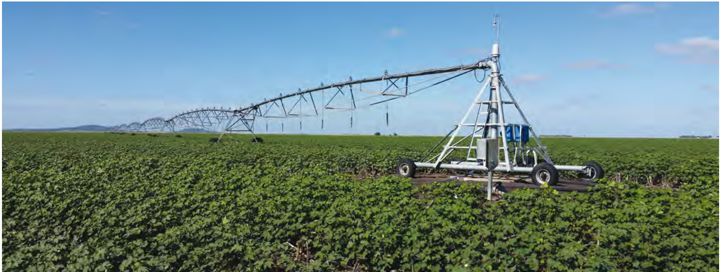
Variable-rate centre pivot irrigation machine on the Darling Downs.
