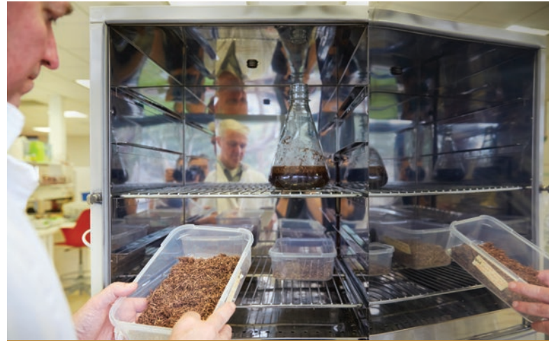
Processing of various straw sources to extract sugars for hydrogen production. (Photo: Nick Cubbin)
