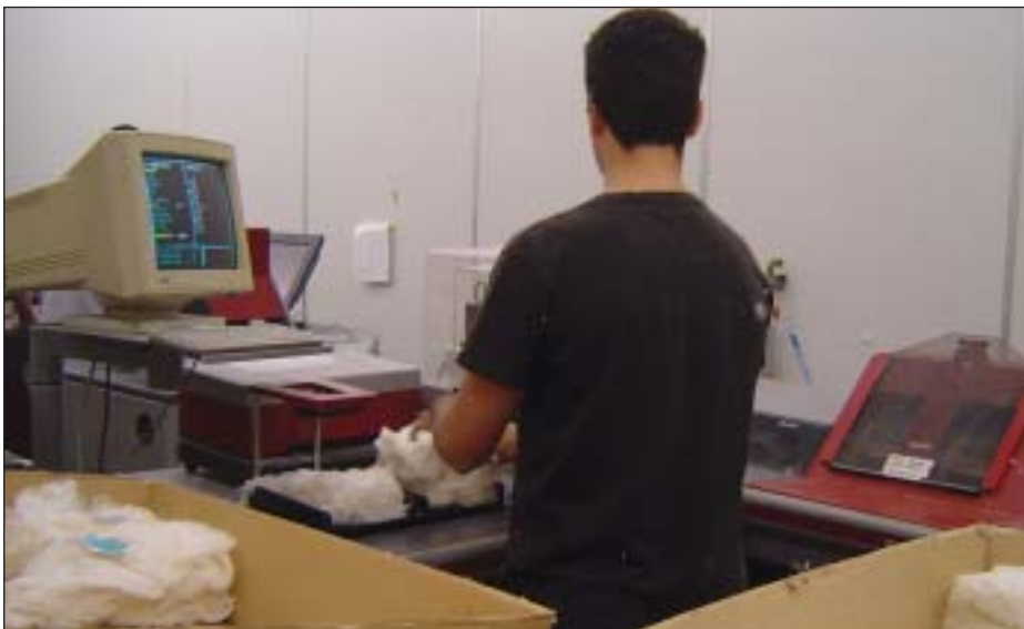
Cotton fibre properties being tested on an HVI instrument.
