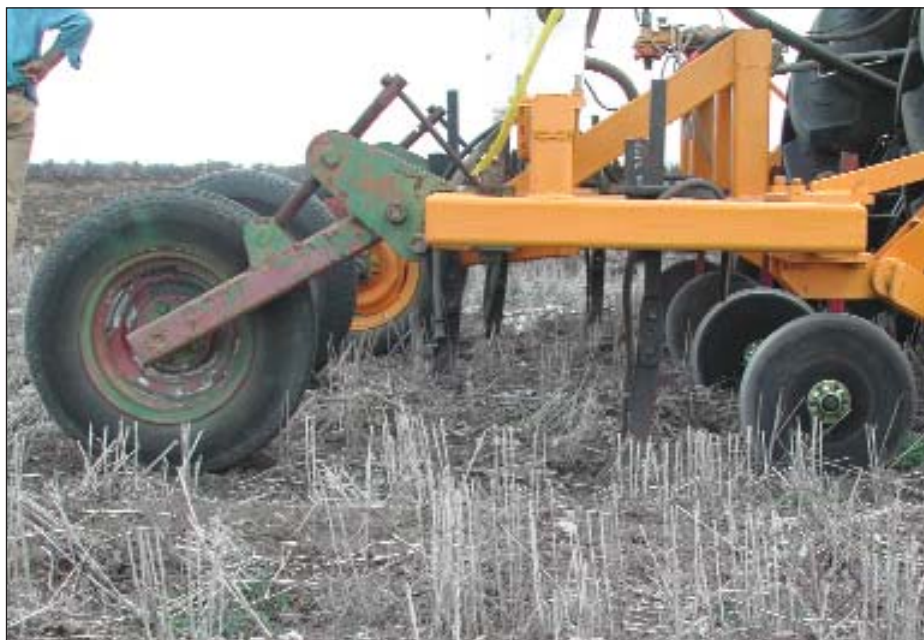
Modified gas (anhydrous ammonia) rig with coulters in front of gas knives
