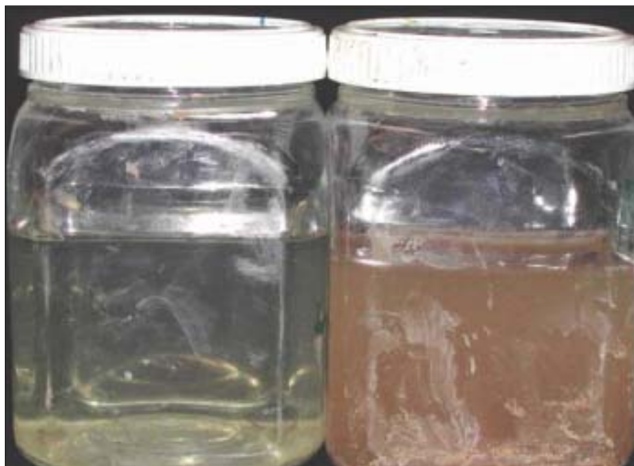
FIGURE 3: Runoff water from plots near Boggabri where cotton was sown either into standing wheat stubble (left) or after wheat stubble (right) was incorporated. Photograph M. Hickman.
