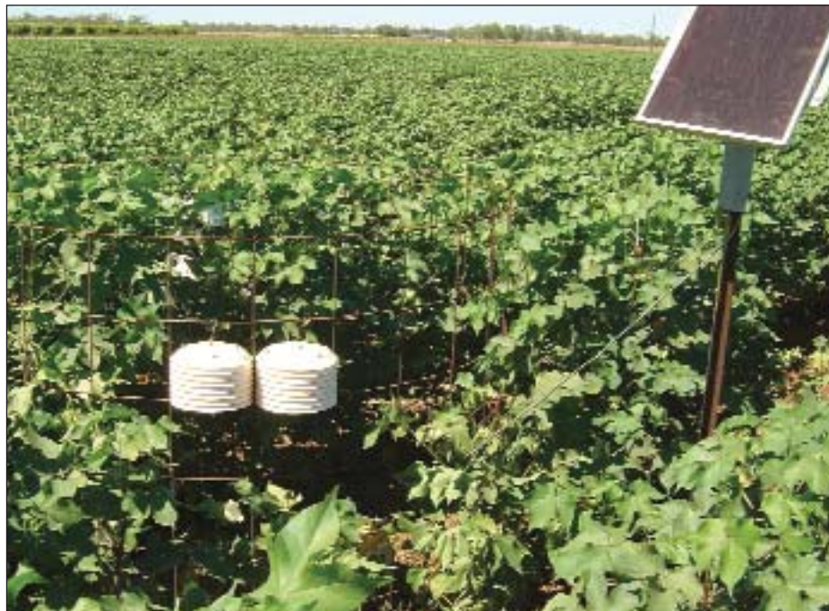
A wallaby proof fence surrounds the temperature data loggers. The solar panel keeps the 12 volt battery charged which powers the time lapse camera.
