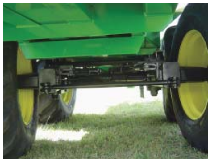
The German-made BPW tandem undercarriage with two metre wheeltrack was built to suit tramline paddock layouts.
