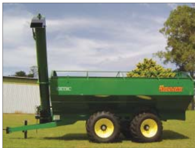
Oztec claims the 24 tonne capacity Tramliner is the first locally-built chaser bin to use the BPW steerable undercarriage.
