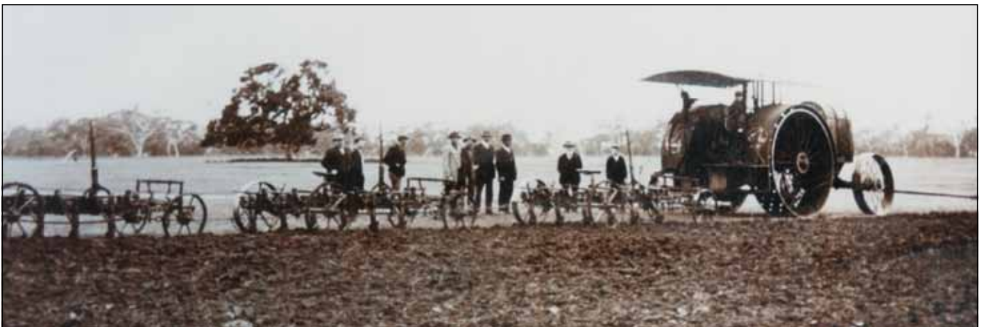
A historic photo of The Big Four operating at the beginning of the twentieth century in the Parkes district. Note the three horse ploughs which the big tractor would have hauled effortlessly. John Deere entered the world of farm tractors with a marketing arrangement of the Big Four with the Transit Thresher Company of Minneapolis which, during that period manufactured The Big Four.
