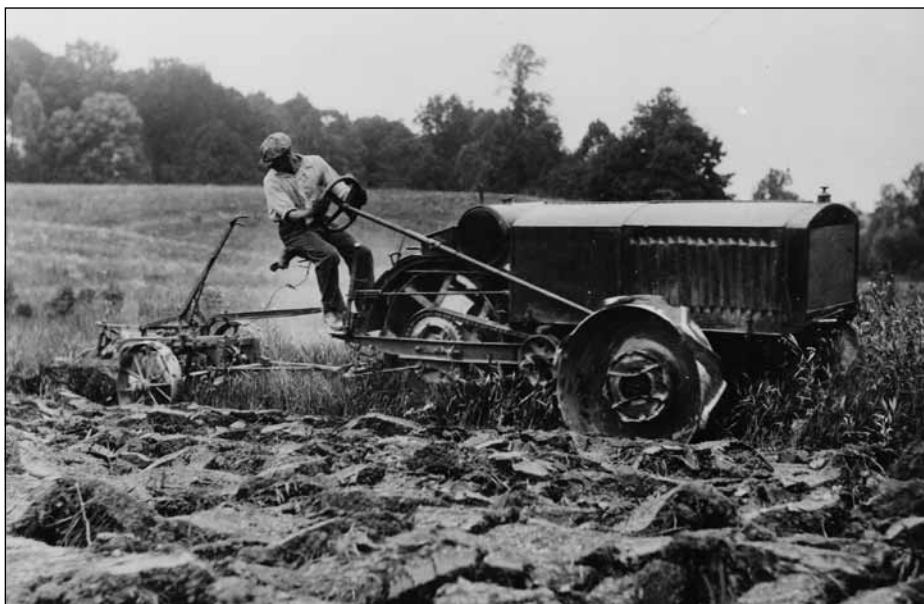
Deere and Co released its second in-house designed tractor in 1916. Note the three-wheel drive configuration. Although a reasonable performer, the cost of production rendered it uncompetitive and only around 200 units were manufactured. At least one example remains in the US and is insured for a figure in excess of one million US dollars. (PHOTO: Courtesy Deere and Co archives)
