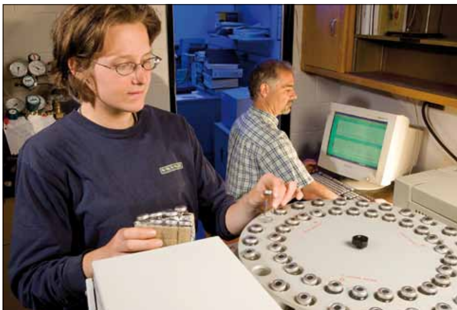
University of Minnesota technician Sonya Ewert (left) and ARS soil scientist Rodney Venterea use a gas chromatograph to determine amounts of greenhouse gases in samples collected from the field. (PHOTO: Stephen Ausmus)
