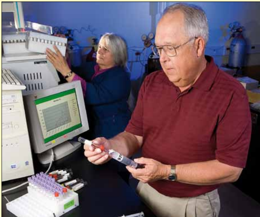
In a nitrogen fertiliser source study, soil scientist Ardell Halvorson (right) and technician Mary Smith prepare gas samples from field sampling for gas chromatograph analysis of nitrous oxide, carbon dioxide, and methane. (PHOTO: Stephen Ausmus)
