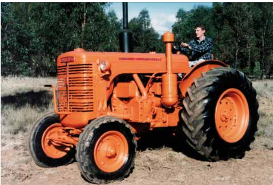
Mathew Puls of Dubbo, NSW is seen here demonstrating his immaculately restored Chamberlain 40KA. Note the horizontally opposed twin cylinder engine which was designed to run on power kerosene fuel, following its initial start on petrol. (PHOTO: IMJ)
