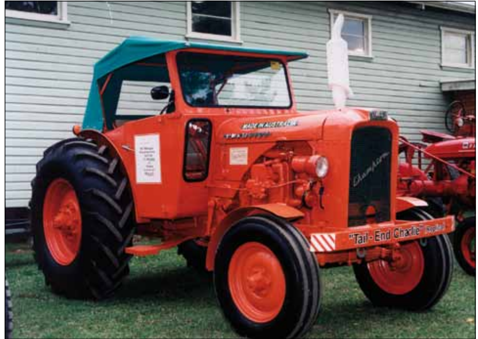
The photo is of a Chamberlain Champion created by the author as a replica of Tail-End Charlie, the famous recovery vehicle which accompanied the 1955 round Australia Redex Trial. It is powered by a four cylinder Perkins 270D diesel engine. (PHOTO: IMJ)
