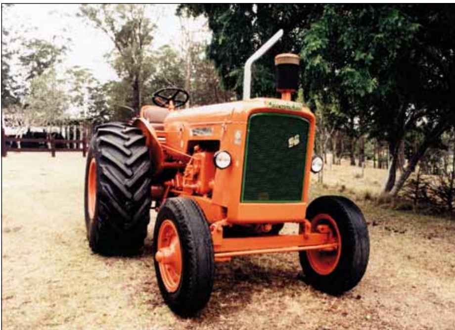
Pictured is the same tractor, clearly showing the soft riding transverse leaf spring front suspension. The tank alongside the engine is in fact the hydraulic reservoir to which is attached the valve control block. In an endeavour to deflect the roar of the two stroke engine, in this example the exhaust pipe has been extended and angled away from the operator. On a still evening, when night ploughing, the distinctive sound of a Super 90 under power could be heard for miles. (PHOTO: IMJ)
