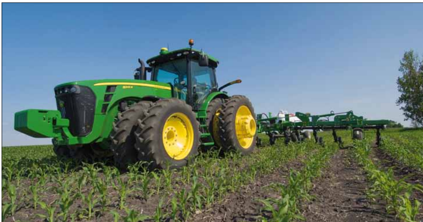
The 8345R is the most powerful row-crop tractor John Deere has ever built – producing up to 345 (257kW) engine horsepower.
