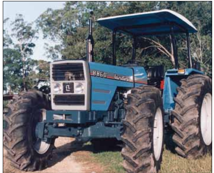
This 1998 Landini 8860 is the author's farm workhorse and is powered by a Perkins 80 HP diesel. It is provided with 24 forward and 12 rear gear ratios. An almost identical tractor was manufactured by Landini at Fabbrico for Massey Ferguson and was marketed as the MF 393 (see text). (Photo IMJ)
