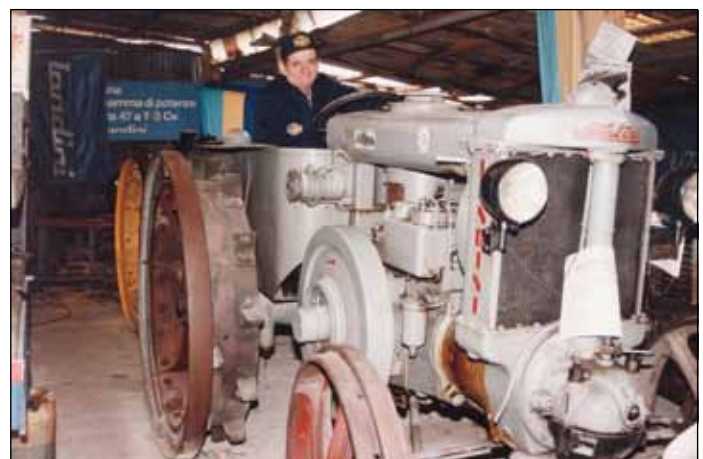
Guido Rondini at the wheel of an 8.5 litre Super Landini which developed 48 HP at 620 RPM. The Super model was produced from 1934 until 1951. (Photo IMJ)
