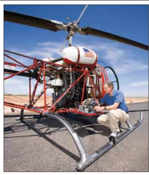
Before takeoff, physical scientist Andrew French prepares camera equipment for airborne multispectral imaging. The data collected is used to estimate crop water use.
