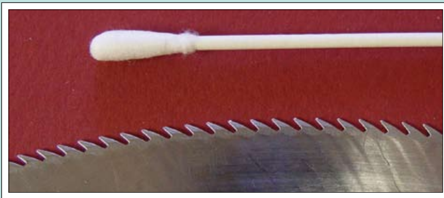
The modern gin stand is capable of producing 15 bales of lint per hour yet it takes an average 20 teeth on a saw to remove enough cotton to make one cotton bud end.
