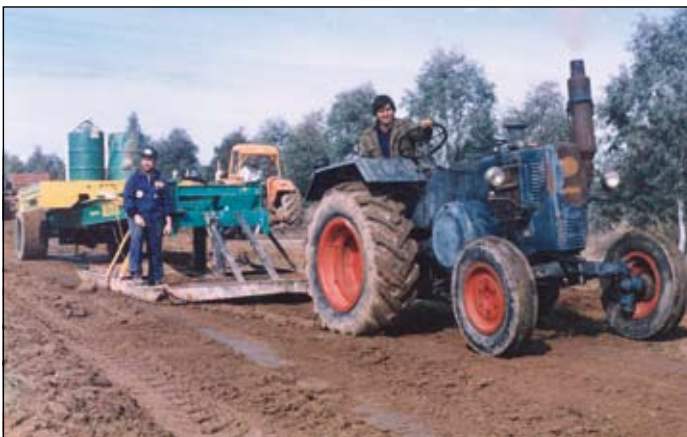
This Lanz Bulldog is equipped with standard cast iron rims. What is not noticeable is the fact that the sheet metal floor of the cockpit has been replaced with three inch cast steel. (Photo C. Galbraith)
