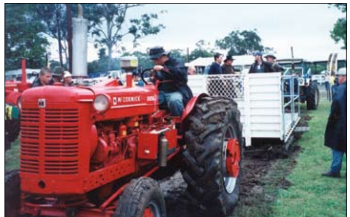
An International McCormick WD6 is fitted with axle weights which extend wider than the rear wheels. At some tractor pulls this would be disallowed. (Photo M. Pettit)
