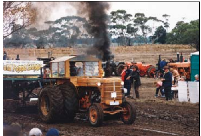
This poor old Chamberlain has been repowered with a doctored 100 hp engine and fitted with dual rears. (Photo IMJ)
