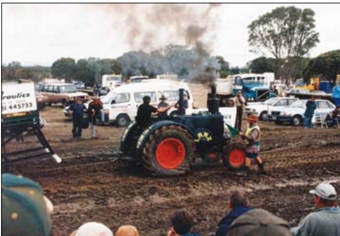
The old Lanz Bulldog is really copping it! Note the flexing of the tyres as it struggles to obtain adhesion. (Photo IMJ)
