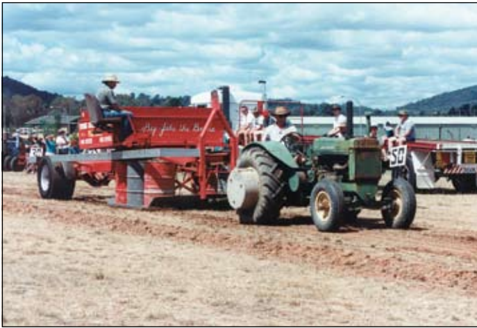
A John Deere AR with grossly heavy concrete counterweights attached to the rear wheels. (Photo IMJ)
