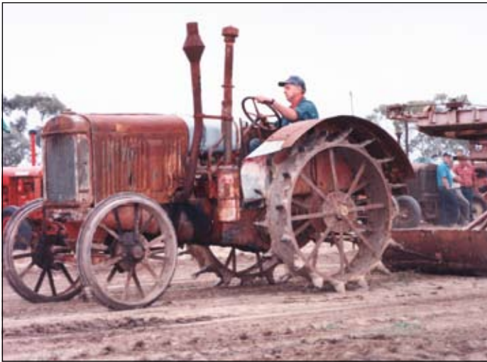
This old McCormick is equipped with steel wheels and lugs. People often mistakenly assume that these lugged wheels will obtain greater traction than if fitted with pneumatic tyres. Nebraska Tractor Test figures prove that in fact the pneumatics obtain a greater grip of the ground. (Photo IMJ)
