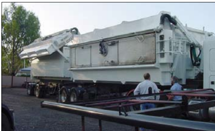
The B-Double with bins that allow you to cart your grain to the terminal and backload with biodiesel.
