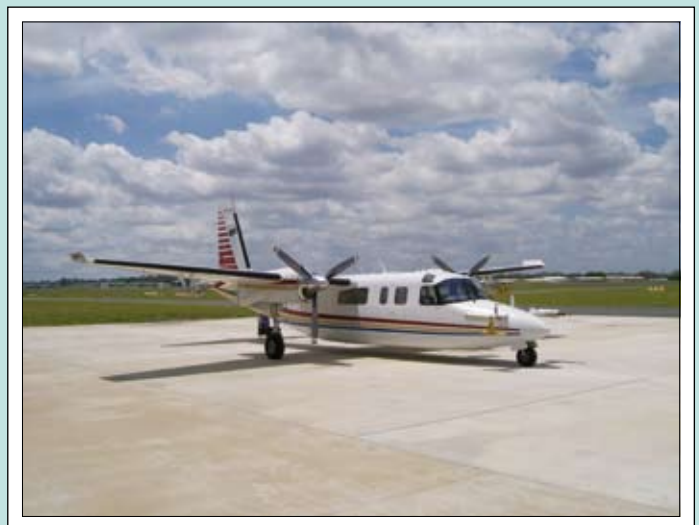
SAWS Aero Commander festooned with cloud droplet, atmospheric and aerosol measuring instrumentation. (PHOTO: US NCAR).
