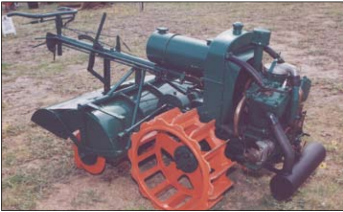
Pictured is a well restored example of a Howard 13 hp rotary hoe, powered by Howard's own water cooled V twin petrol engine. The unit is equipped with a three forward and one reverse speed gearbox. It is owned by Allan and Kim Dhu of Bunbury, WA. (Photo IMJ)
