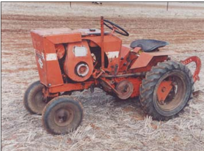
The Howard 2000 was introduced to the range in 1962 and was powered by a 12 hp single cylinder air cooled petrol engine. The rear implement was raised and lowered manually by the hand lever on the left side of the tractor. This particular unit competed in the world championship winning event Plough and be Counted 2, held at Cootamundra, NSW (Photo IMJ)
