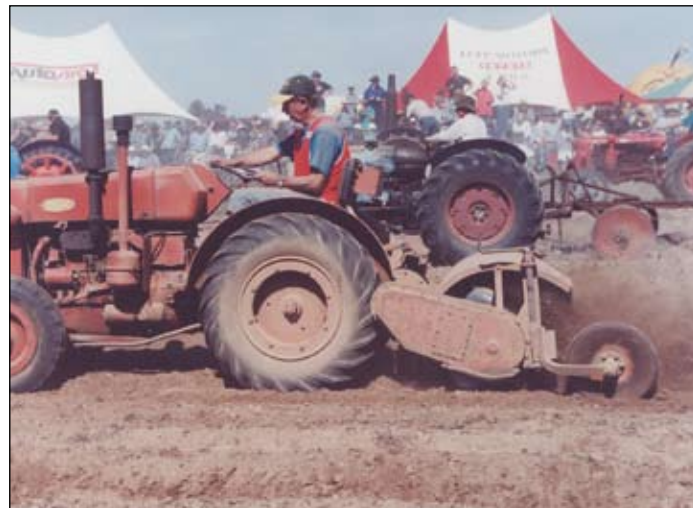
The Howard DH 226 succeeded the DH 22 in 1952. It was equipped with a Le Roi four cylinder petrol engine of 35 hp. The rotary hoe was raised and lowered hydraulically. This particular unit was demonstrated at Yass during the successful Plough and be Counted World Record Attempt for the greatest number of tractors ploughing at the one time in the one paddock. (Photo IMJ)
