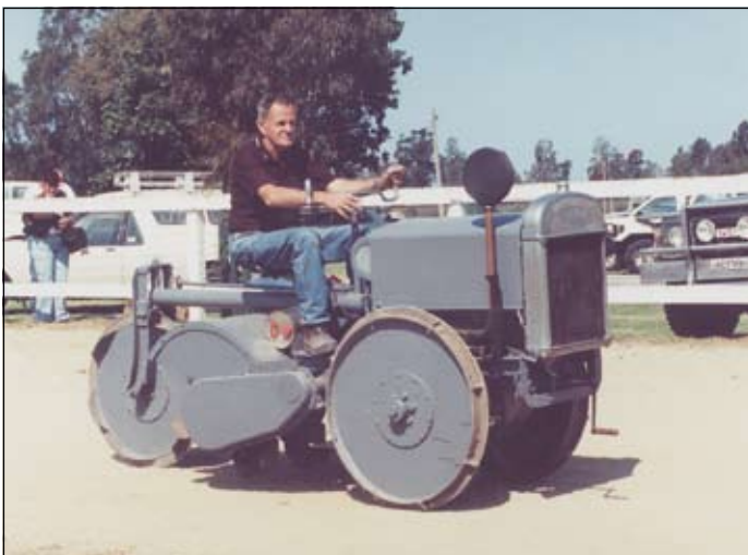
The Howard 16 was introduced in 1928. It was powered by a Morris Commercial 16 hp petrol engine. Pictured is one of the few remaining examples and was exhibited at the 2006 Rusty Iron Rally. (Photo IMJ)
