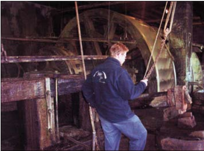
Clearly illustrated are the two water wheels. A closer scrutiny to the left of the controller is one of the iron clad wheels with the steel cams, which actuate the hammer (to the controller's right) at 150 strokes per minute. (Photo IMJ)
