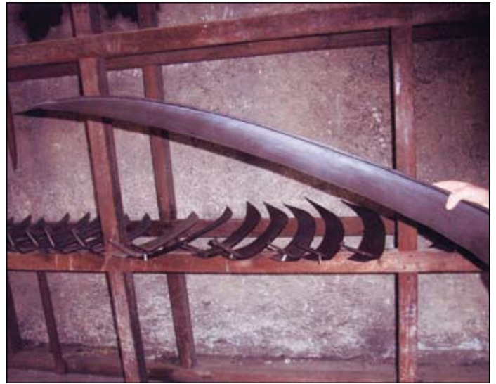
The finished article. A beautifully crafted razor sharp scythe blade. Various shapes of blades are displayed on the rack behind. (Photo IMJ)
