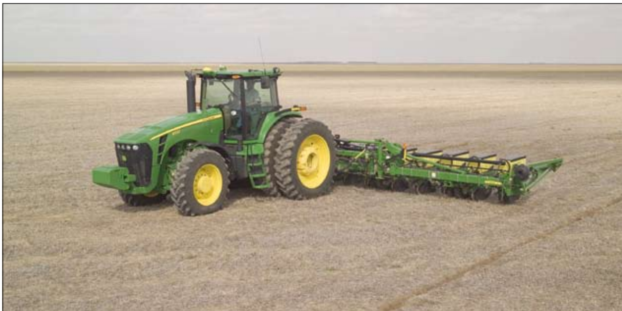
A 1720 MaxEmerge Plus planter coupled with a 8530 tractor.
