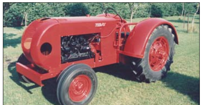
A springtime photo of the Friday, clearly showing the big six cyl Chrysler engine which, without a governor, is capable of propelling the sleek tractor at speeds restricted only by the nerves of the operator. (Photo R. Rosenboom)
