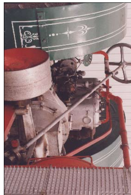
The engine of the Galloway is a 4 cyl side valve Dart with a 4.5 x 5 inch bore and stroke, developing 20 bhp. The gearbox is located between the engine and radiator and provides one forward and one reverse gear. The engine is cranked from the rear. (Photo IMJ)
