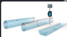
Measure: Open channel, full or partially full pipe flows with one AgriFlo Series 3.
