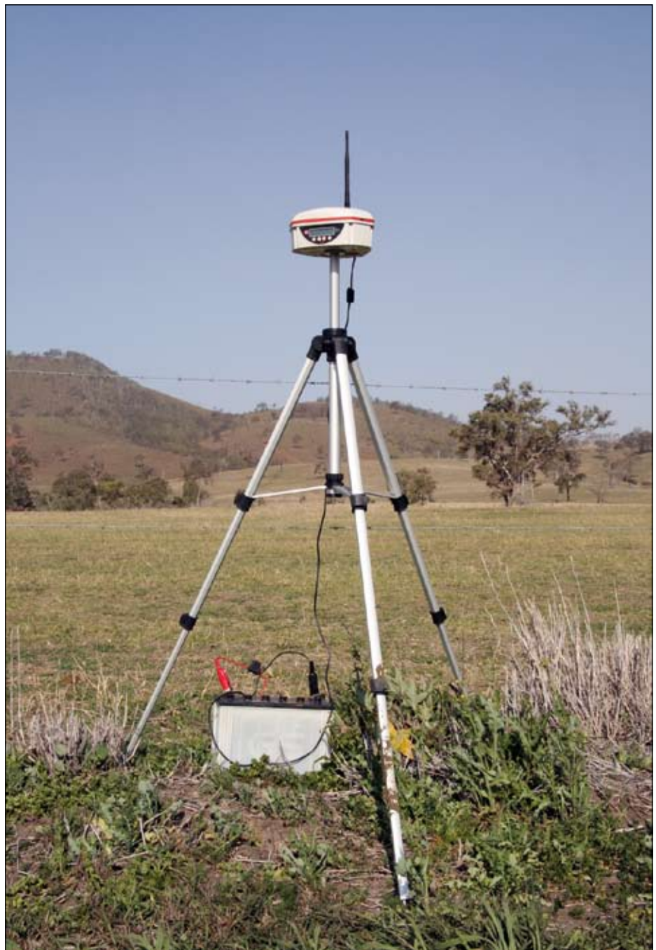
The battery powered mojoRTK test site.
