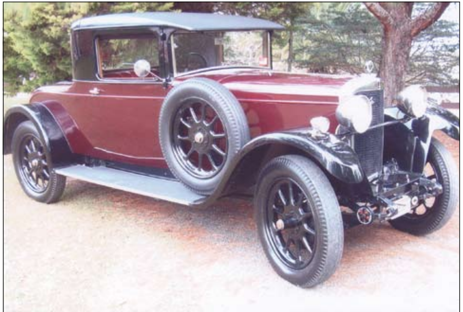
This 1928 Talbot 14/45 is believed to be the only entirely original AD version of a Doctor's Coupé coachbuilt by Damyon Bros. remaining in the world. It is powered by a six cylinder ohv engine which develops 45 bhp and has a maximum speed of 106 kph but cruises comfortably at 85 kph. (Photo IMJ)
