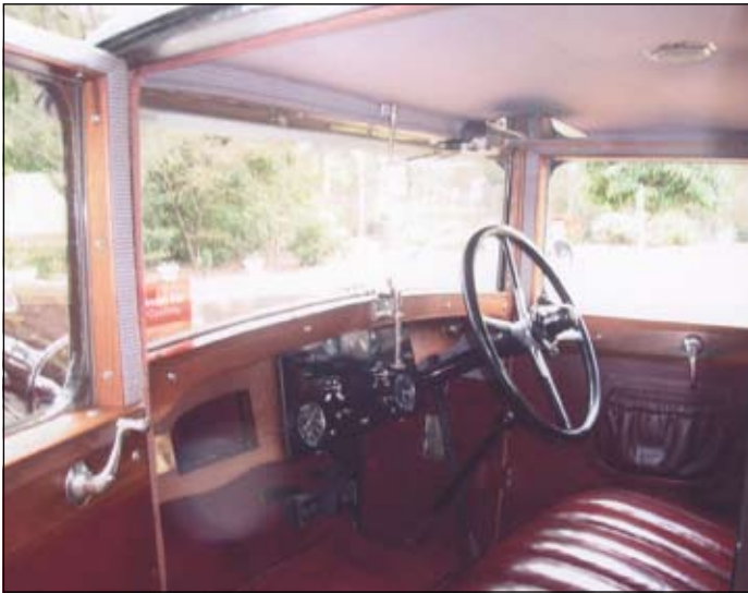
The lush interior trim is rich Connolly leather, deep Wilton carpet and solid oak. The front windscreen opens forward and provides a good flow of cool air in hot weather. The centre of the steering wheel accommodates turning indicators, high low beam dipper, hand throttle and Klaxon horn button. (Photo IMJ)
