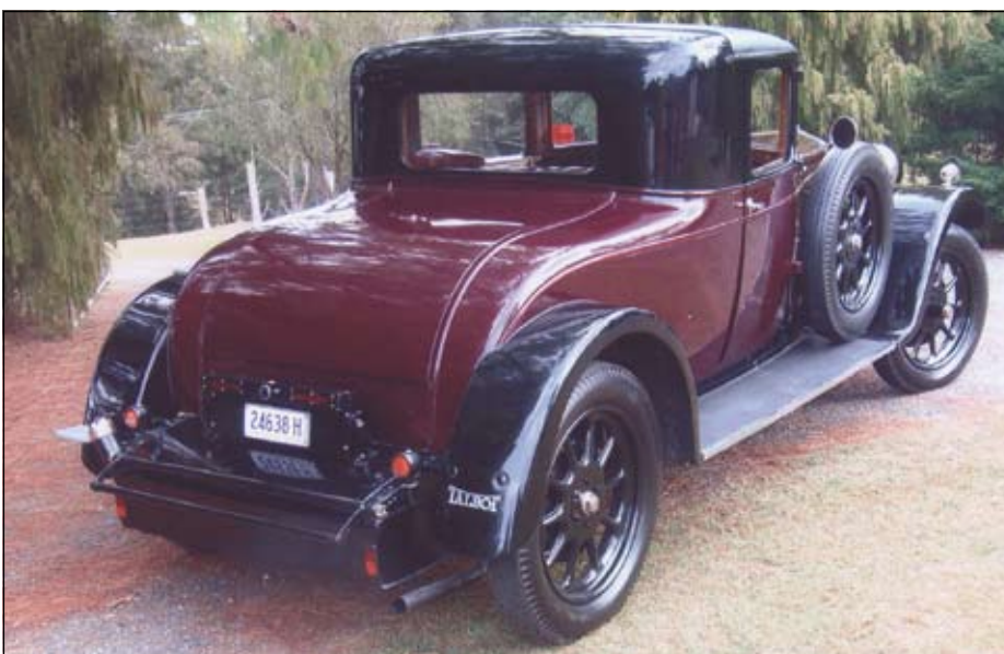
The boot at the rear is immense, presumably to accommodate a visiting Doctor's paraphernalia. The rear fuel tank holds 60 litres. The fuel is drawn to the carburettor by a vacuum system. Interestingly, the Talbot 14/45 was the first car ever to be fitted with flashing turning indicators — and all that in 1928. (Photo IMJ)
