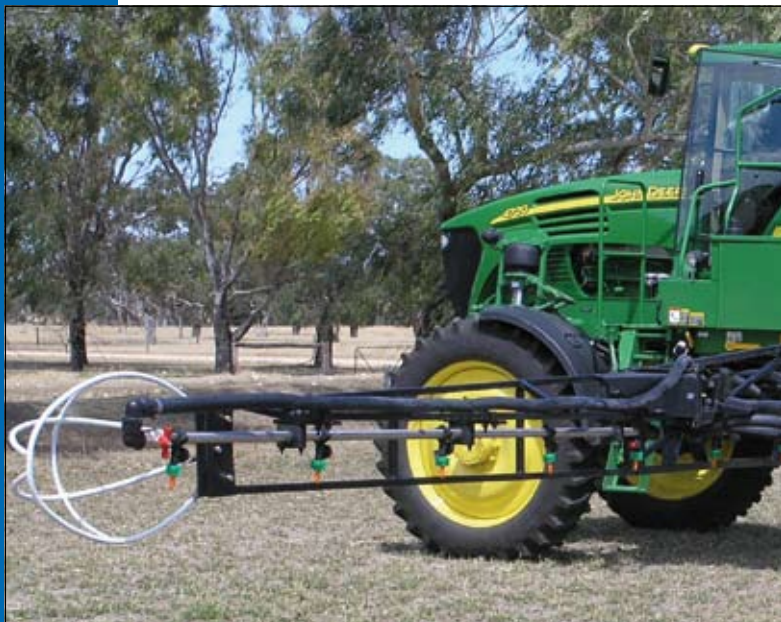
An example of manual boom recirculation plumbing.
