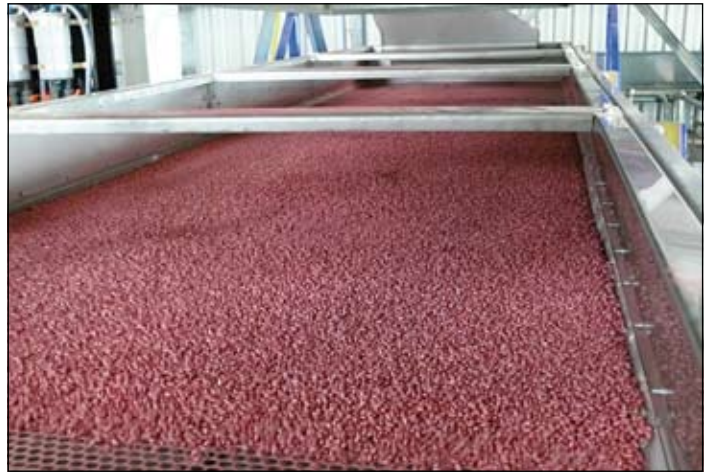
Some of the new CSD seed treatment system — chemical control modules (left) and treated seed on the gravity table.
