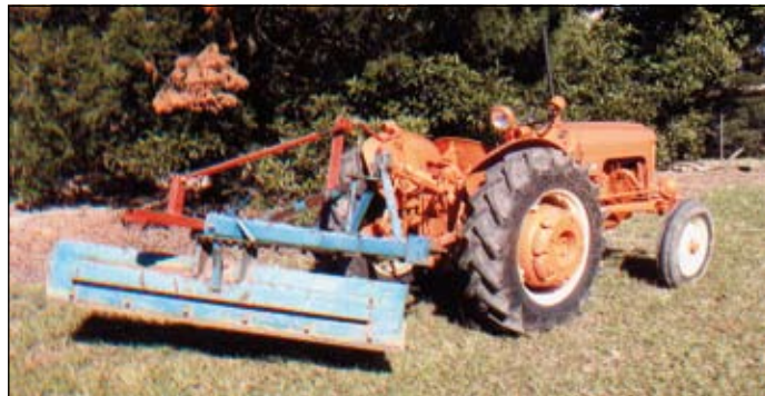
The vintage BMC Mini tractor fitted with a Berends rear grader blade. (Photo IMJ)
