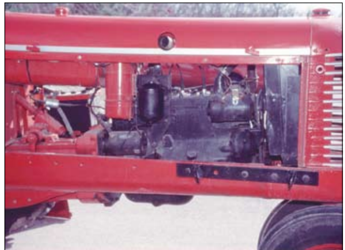
With the side panels removed, easy access is provided for servicing the Graham Page six cylinder side valve engine. (Photo IMJ)
