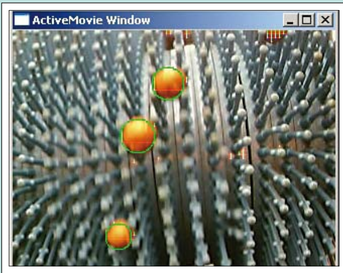
ROC can identify and analyse macadamia nut density on picker bristles to calculate tree yields. Another side scanning camera locates and identifies individual trees to yield per tree.
