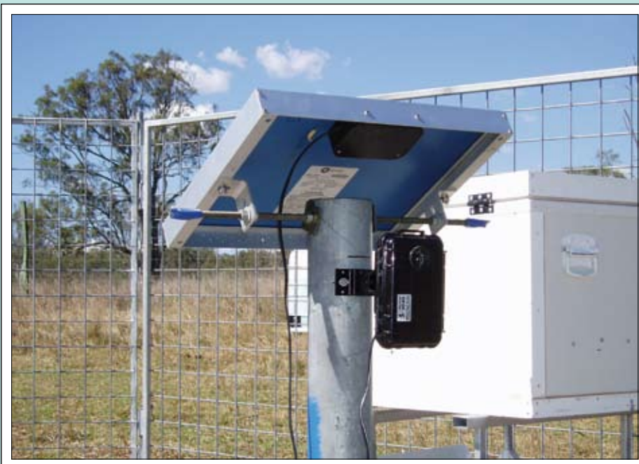
The ROC features rugged portability, low battery drain and remote reporting facilities.
