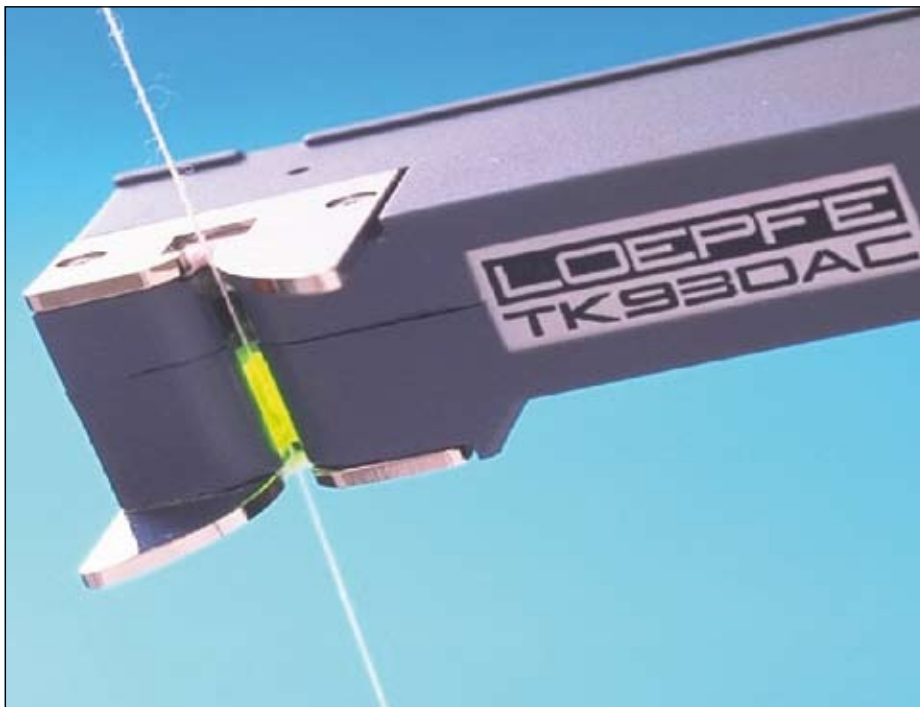
Yarn clearer to remove foreign matter from yarn in winding and open end spinning. (Photo courtesy of CSIRO Textile and Fibre Technology)
