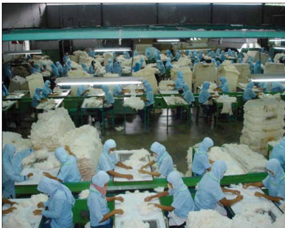
Manual removal of contaminants from cotton before release to spinning mill. (Photo courtesy Apac Inti)
