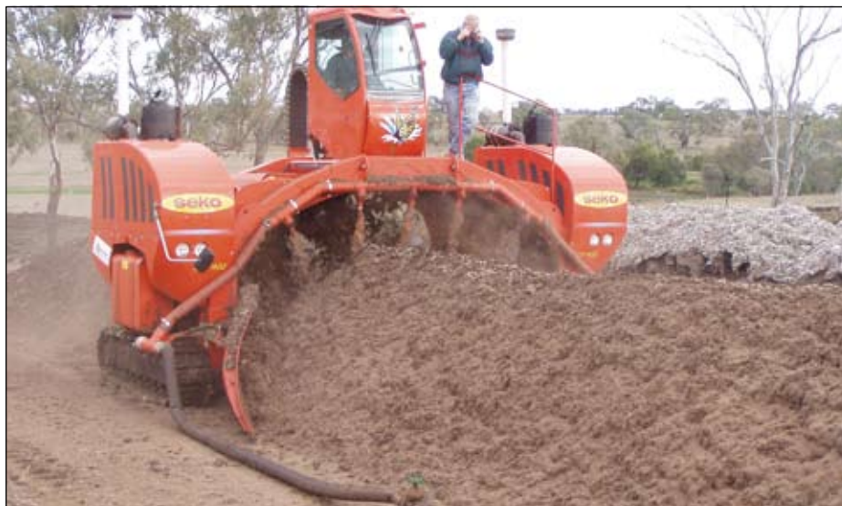
A windrow machine turns cotton gin trash windrows while simultaneously wetting the material with effluent as part of a trial at a piggery west of Toowoomba.
