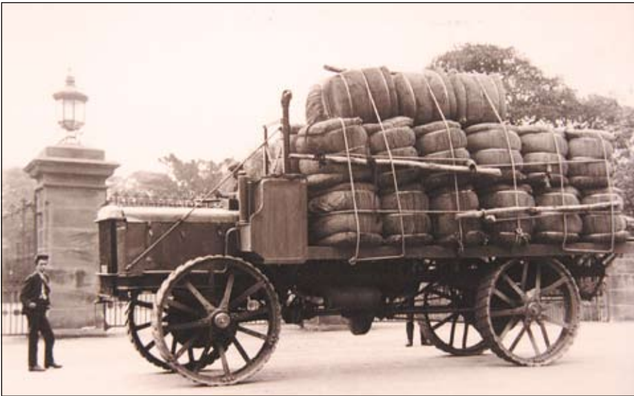
This photo taken in 1910 is of a Caldwell Vale Rough Terrain Road Tractor loaded up with bales of wool. These big transporters had a top speed of six miles per hour. (Photo IMJ archives).
