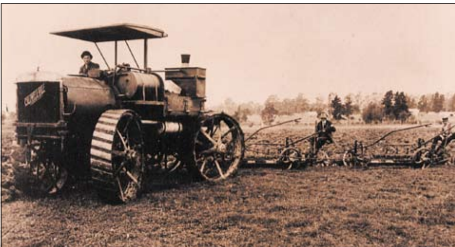
A 1910 photo of the 80 hp Caldwell Vale in action. Note the four wheel steer, also the additional cooling tank mounted on the rear of the tractor, suggesting that the front radiator alone was insufficient to maintain a normal working temperature for the engine. (Photo IMJ archives).
