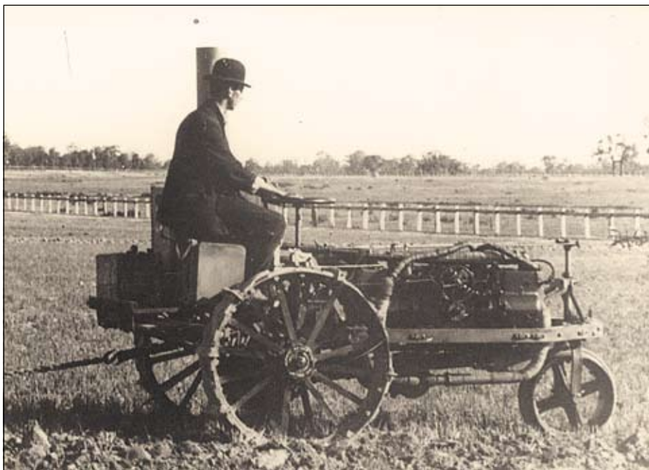
A 1910 archival photo of an Ivel under test at the Yanco Agricultural College, New South Wales. The bonnet has been removed. This was a common practice, as the two cylinder engine was prone to overheating. Also pressure was created in an oily discharge around the engine if the bonnet was in place. (Photo courtesy The Manning Valley Historic Museum, Wingham).
