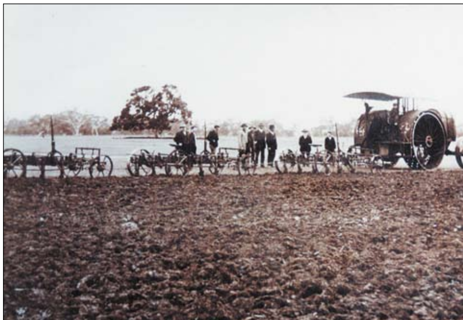
An Emerson Brantingham Big Four operating in central New South Wales. Note the three ploughs which the big tractor would handle with ease. (Photo courtesy Pioneer Park Museum, Parkes, New South Wales).
