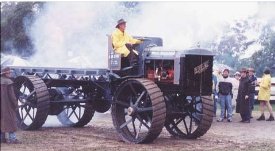
A contemporary photo of a fully restored Caldwell Vale, being demonstrated at the 2004 Rusty Iron Rally. The restorer and operator is Reg Schuster. The engine had just been started and the cloud of smoke from the exhaust disappeared as the engine warmed up. (Photo IMJ).
