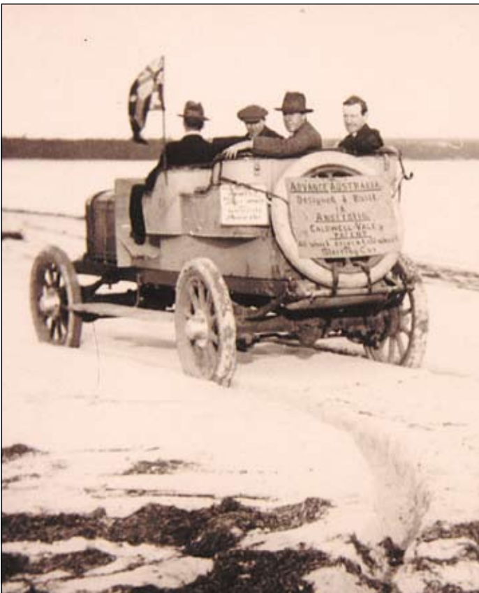
Pictured is the world's first four wheel drive, four wheel steer, touring car. This Caldwell Vale innovation is being tested at the Cronulla sand hills, circa 1913. (Photo IMJ archives).
