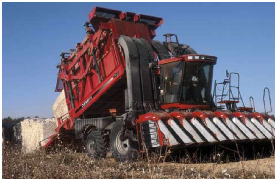
The Case IH Module Express 625 is the first commercial cotton picker with the ability to build modules while harvesting.
