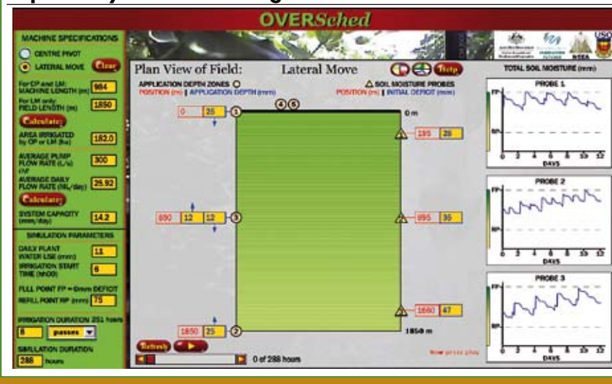
FIGURE 2: Predicted soil moisture under a lateral move machine — you can go back and change your application depth to try different strategies
