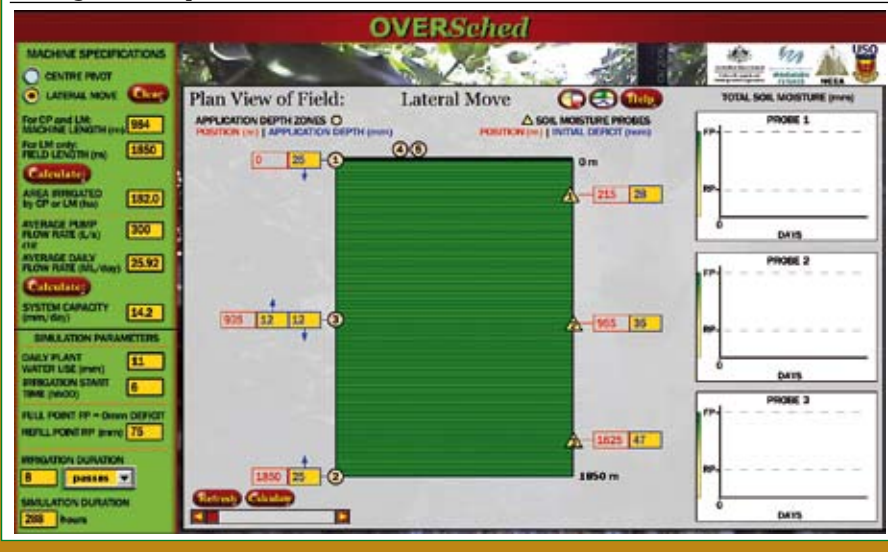
FIGURE 2: Predicted soil moisture under a lateral move machine — you can go back and change your application depth to try different strategies
